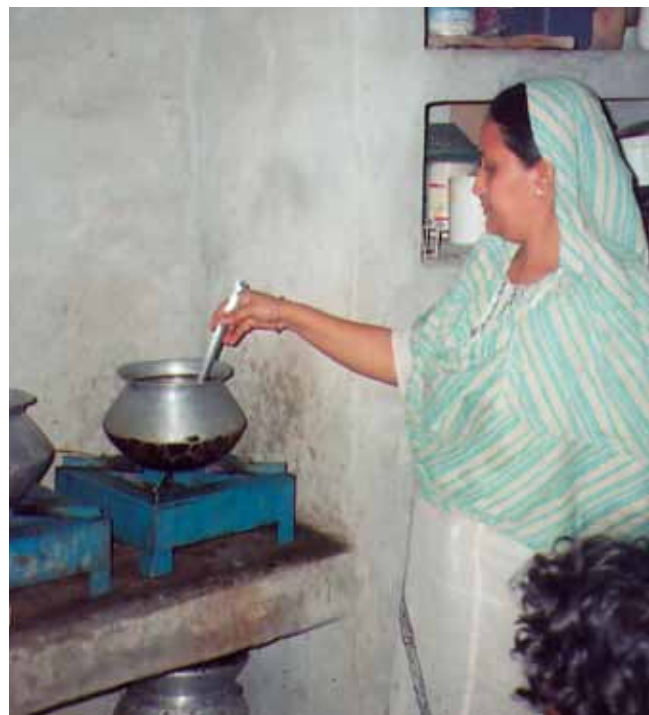
Biogas cooking stoves, which use fuel generated from the anaerobic digestion of waste cow dung, are transforming rural Bangladesh. A family with two cows can generate enough biogas to meet its daily cooking needs
